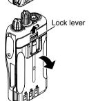
To remove the battery pack, push the lock lever up, then pull the battery pack away from the transceiver.
