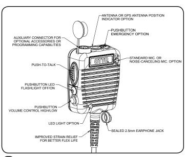
Turn the radio on and operate it as explained in the operating instructions supplied with the radio. Installing the speaker microphone (1) bypasses the radio's speaker and routes the speaker output to the speaker microphone and (2) disables the radio's microphone and enables the speaker microphone. To enable the microphone, press the large PTT actuator located on the side of the speaker microphone.
