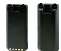
BP-288 Li-ion 7.2 V 2200 mAh (min.) 2350 mAh (typ.) Waterproof BP-289 Battery case 6 × LR6 (AA). Water resistance
